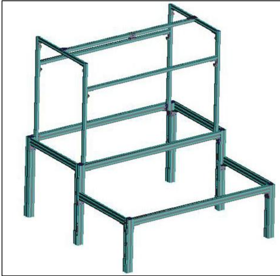
Figure 8: CAD Drawing of Aluminum Frame Used to Support the Rig
