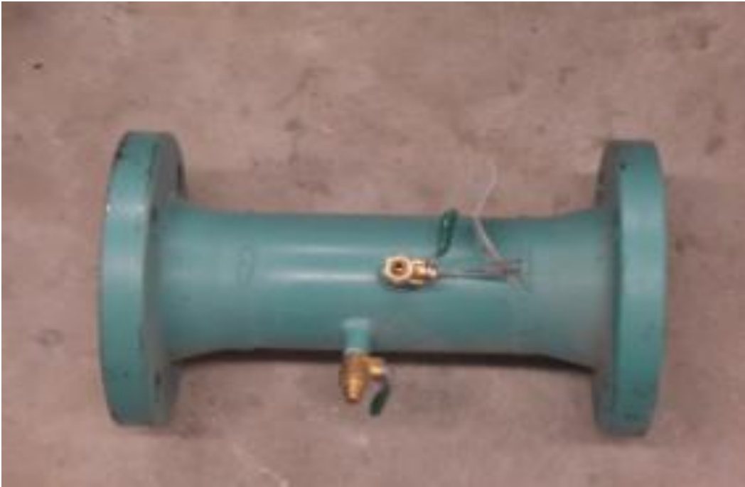
Figure 15: Venturi Meter Used to Measure Flow Rate
